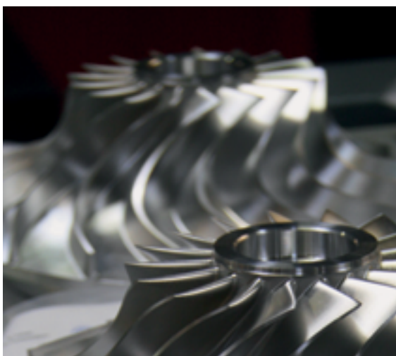
Aerodynamic performance is determined by shape of the blades and tip speed.
