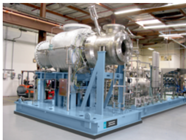
A turboexpander for cryogenic hydrocarbon separation.
