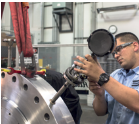
A turboexpander is assembled for a hydrostatic test.
